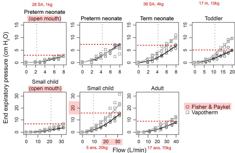
**Fig. 2.** Lung model end-expiratory pressure or PEEP representing simulated alveolar pressure at baseline (no high-flow nasal cannula) and pressure at different flows provided with the Optiflow and Precision Flow high-flow nasal cannula systems. Individual data points are shown for each measurement of pressure, fitted with locally weighted scatterplot smoothing curves. Gray vertical lines represent the change point where a nonlinear relationship between flow and pressure is observed.
